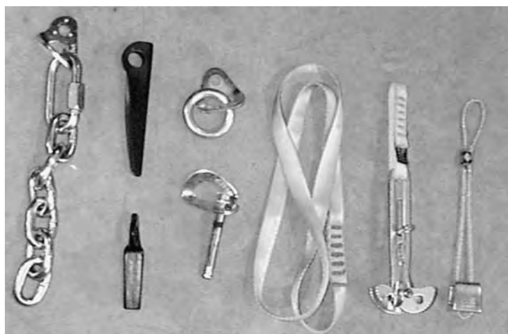
Figure 1—Anchor types from left to right: chain for rappelling, pitons, rappel ring, hanger with expansion bolt, nylon sling, and two types of removable climbing protection (cam and nut). Photo courtesy of Christopher Jones.
